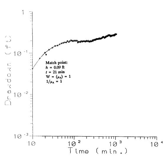
$T = QW(\mu_A) = \frac{3.67 \text{ gpm}}{4\pi h} = \frac{1440 \text{ min}}{4\pi (0.09 \text{ ft})} = \frac{1 \text{ ft}^3}{1 \text{ d}} = 625 \text{ ft}^2/\text{d}$
