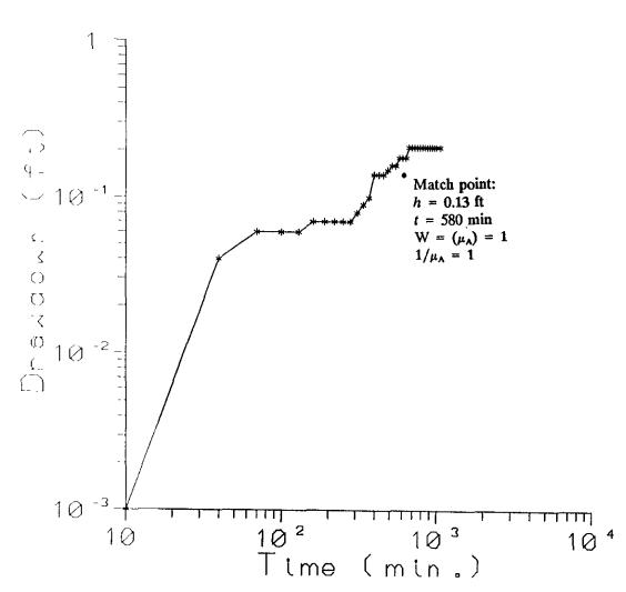
T = QW( $\mu_A$ ) =  $\frac{3.67 \text{ gpm}(1)}{4\pi h}$   $\frac{1440 \text{ min}}{4\pi (0.13 \text{ ft})}$   $\frac{1 \text{ ft}^3}{1 \text{ d}}$  = 433 ft<sup>2</sup>/d
