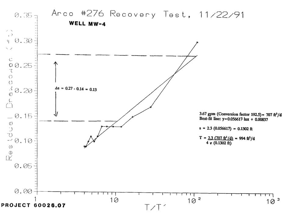
RESIDUAL DRAWDOWN/NORMALIZED TIME WELL MW-4 (SEMI-LOGARITHMIC) PLOT DI ATE 20
