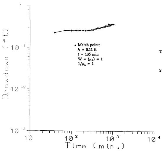
$T = \frac{OW(\mu_A)}{4\pi h} = \frac{3.67 \text{ gpm}}{4\pi (0.11 \text{ ft})} = \frac{1440 \text{ min}}{1 \text{ d}} = \frac{1 \text{ ft}^3}{7.48 \text{g}} = 511 \text{ ft}^2/\text{d}$
