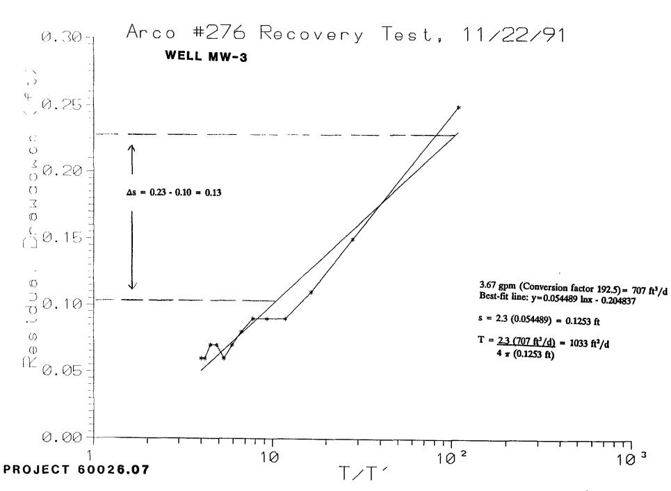
RESIDUAL DRAWDOWN/NORMALIZED TIME WELL MW-3 (SEMI-LOGARITHMIC) PLOT PLATE 10
