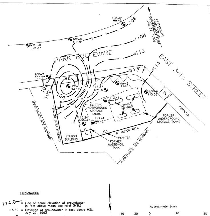
RW-1 = Groundwater recovery well (RESNA, 10/92) MW-10 = Groundwater monitoring well (RESNA, 04/90, 07/90, 08/91, and 06/92)
