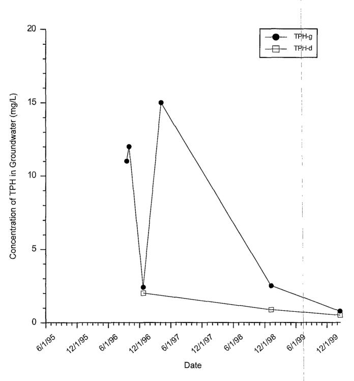
Note: Plotted data does not include diesel concentration of 330 mg/L detected on 6 September 1996 during first sampling event after installation of MW-4.
