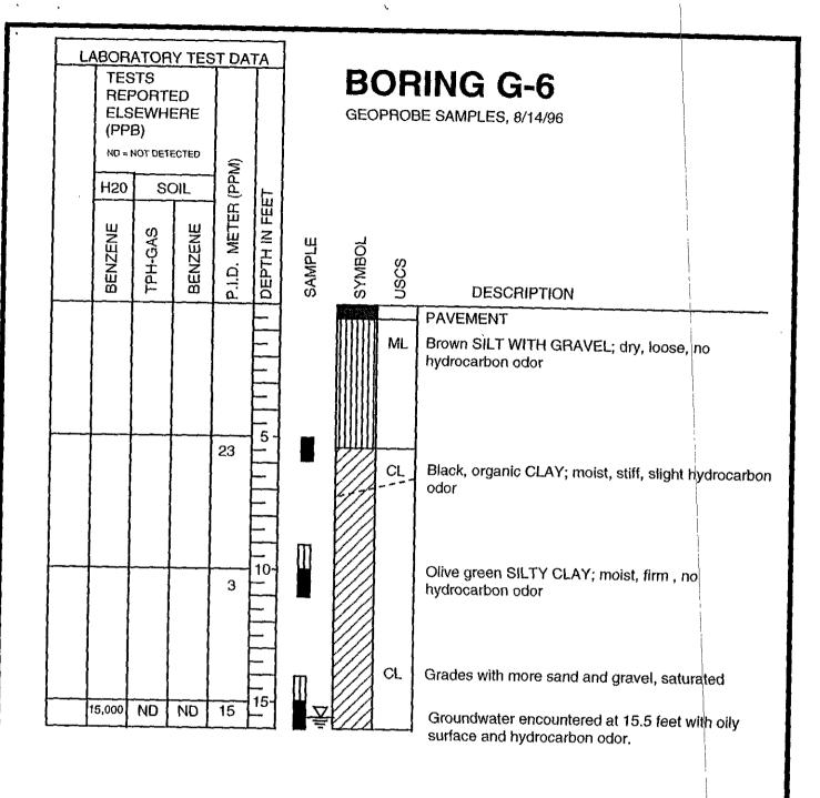
BORING COMPLETED AT A DEPTH OF 16 FEET ON 8/14/96 GROUNDWATER ENCOUNTERED AT A DEPTH OF 15.5 FEET. BACKFILLED WITH HYDRATED BENTONITE.
