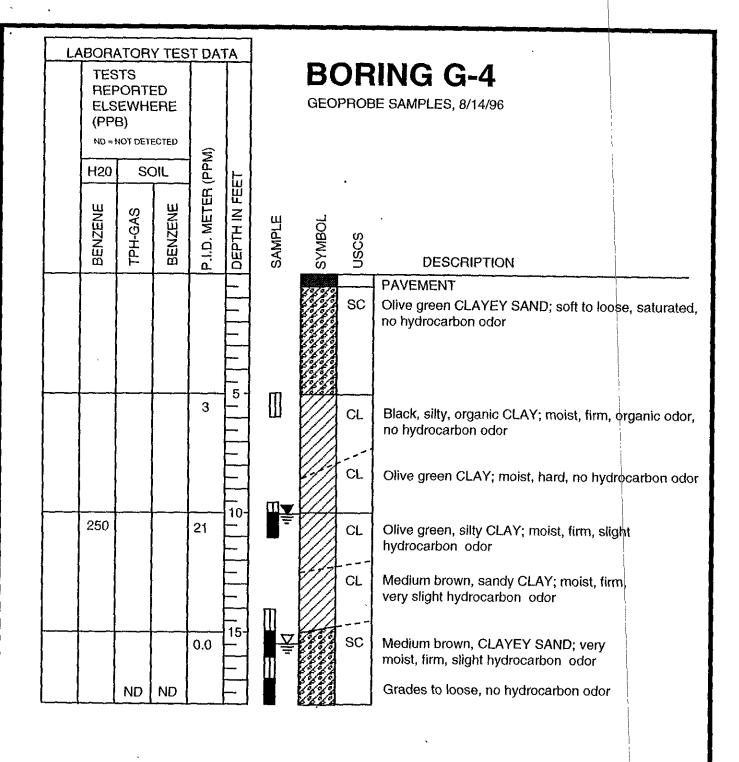
BORING COMPLETED AT A DEPTH OF 22 FEET ON 8/14/96. GROUNDWATER ENCOUNTERED AT A DEPTH OF 15.5 FEET. BACKFILLED WITH HYDRATED BENTONITE.
