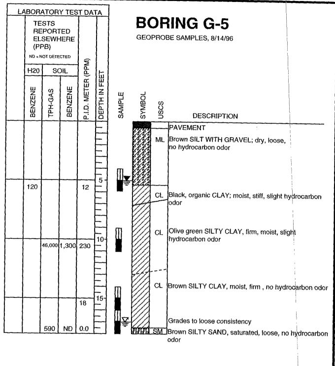
BORING COMPLETED AT A DEPTH OF 18 FEET ON 8/14/96 GROUNDWATER ENCOUNTERED AT A DEPTH OF 17 FEET. GROUNDWATER STABILIZED AT A DEPTH OF 5 FEET. BACKFILLED WITH HYDRATED BENTONITE.
