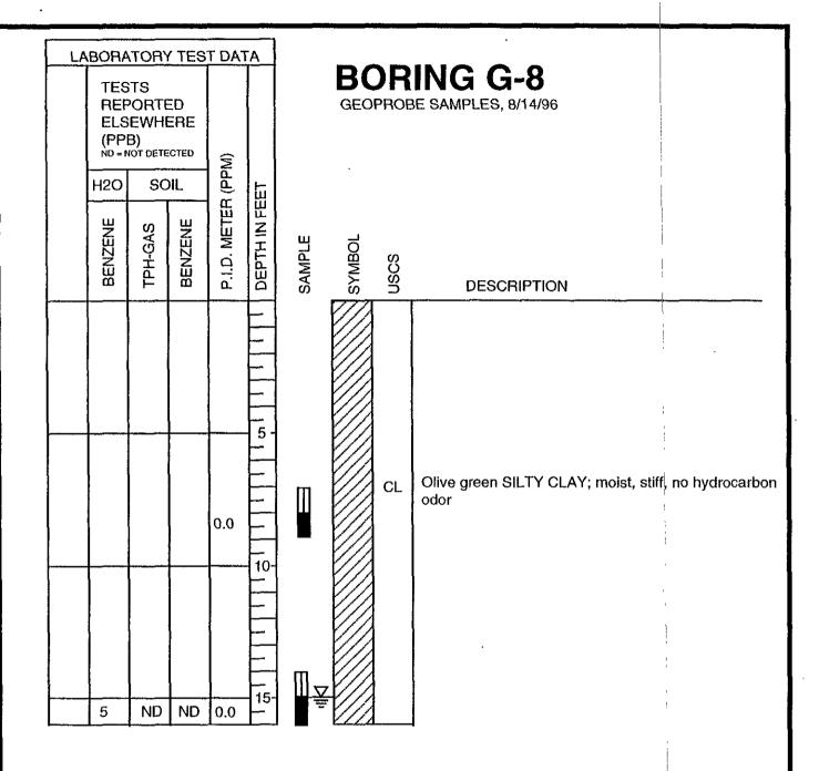
BORING COMPLETED AT A DEPTH OF 16 FEET ON 8/14/96. GROUNDWATER ENCOUNTERED AT A DEPTH OF 15 FEET. BACKFILLED WITH HYDRATED BENTONITE.
