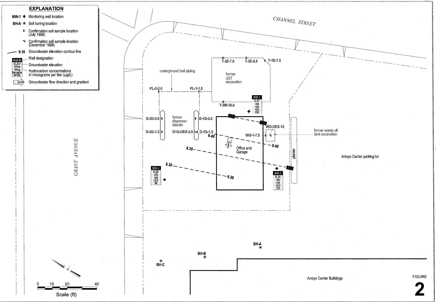
Groundwater Elevation Contour and Hydrocarbon Concentration Map
