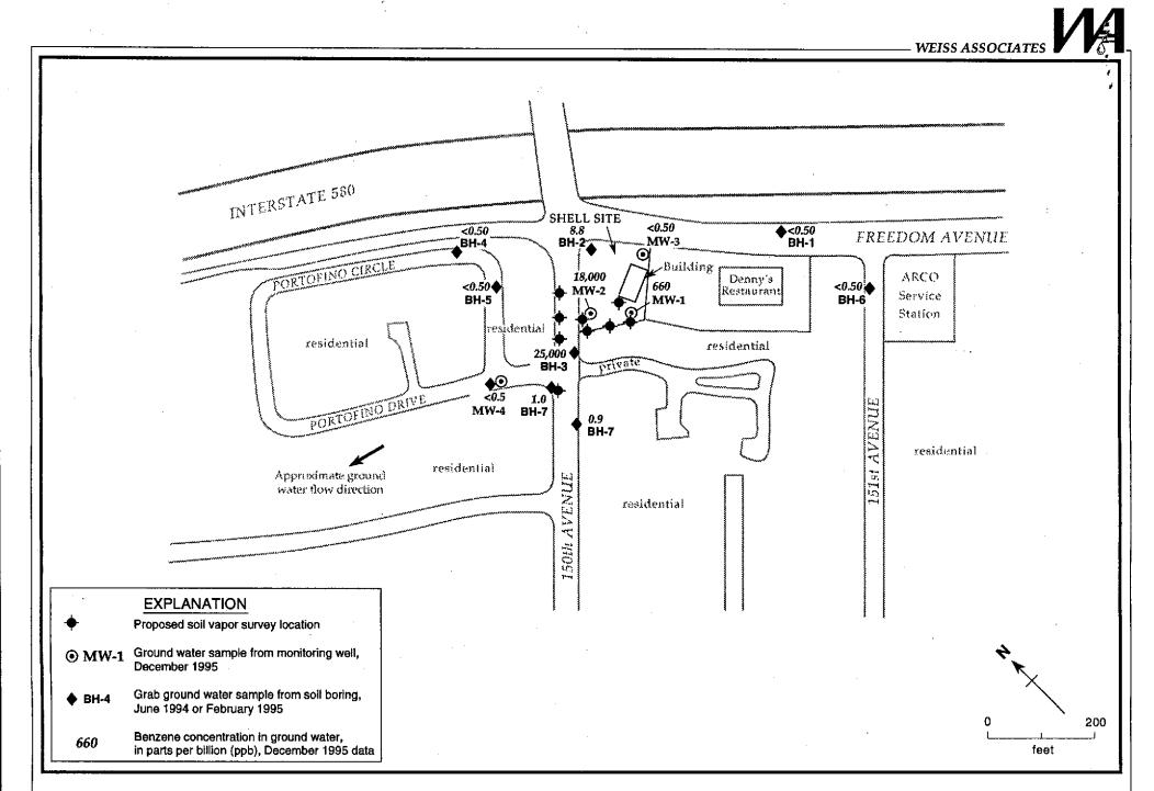
Figure 1. Proposed Soil Vapor Sample Locations - Shell Service Station WIC #204-6852-1404, 1784 150th Avenue, San Leandro, California
