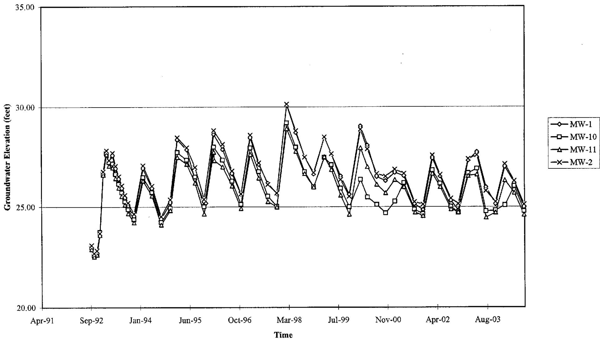
Groundwater Elevations vs. Time
