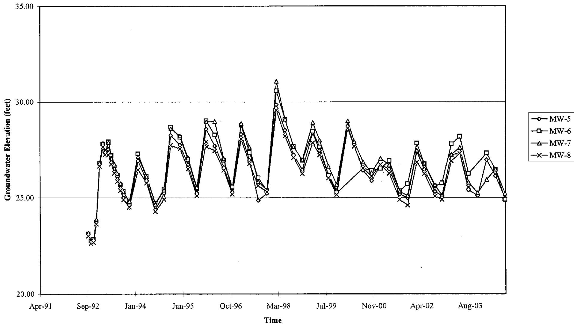
Groundwater Elevations vs. Time
