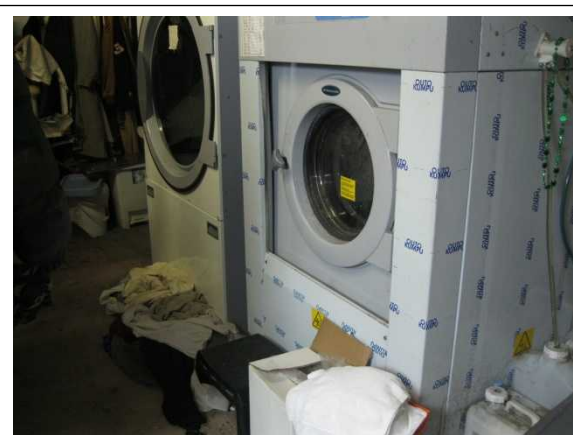
33. Current non-chemical drycleaner machine
