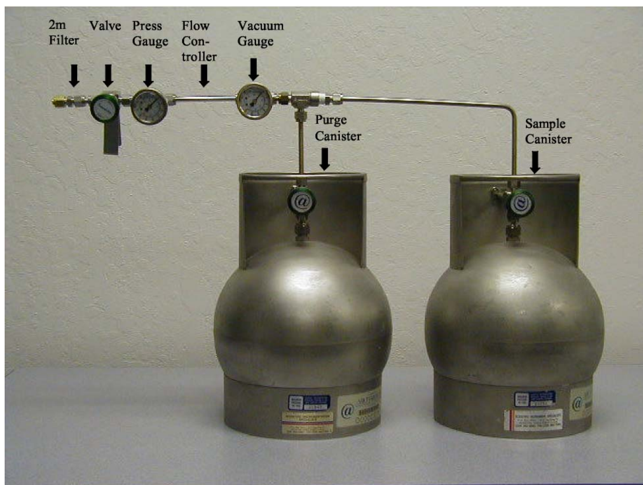
Figure 10. Typical Soil Gas Sample Collection Manifold
