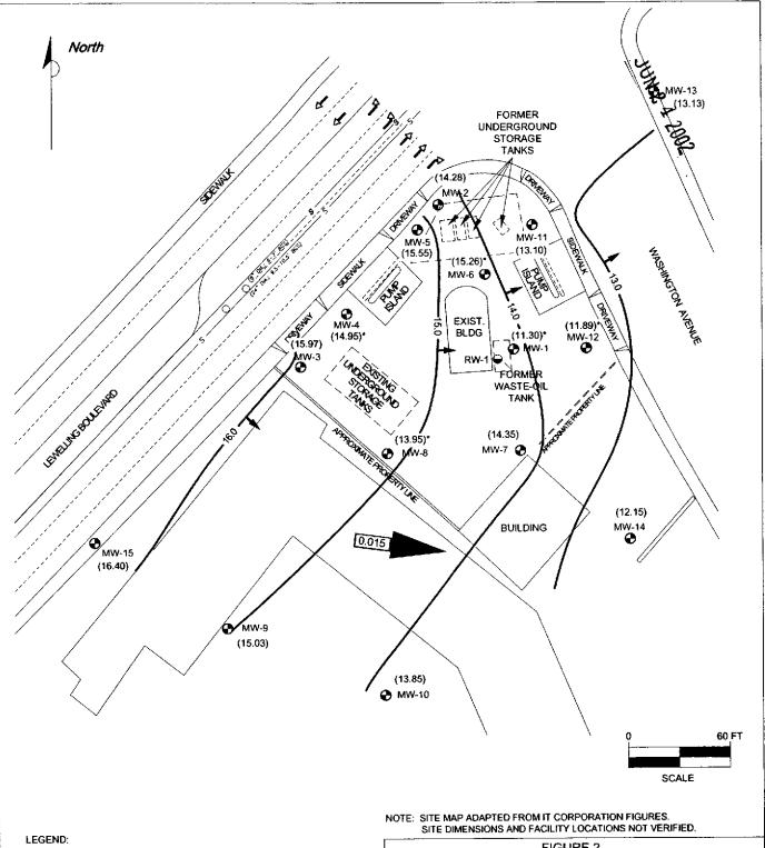
♠ MW-1 MONITORING WELL LOCATION SOIL VAPOR EXTRACTION WELL LOCATION GROUND WATER ELEVATION IN FEET ABOVE MEAN (14.28)SEA LEVEL (MSL) WATER TABLE CONTOUR IN FEET ABOVE MSL **— 13.0 — GROUND WATER FLOW DIRECTION** APPROXIMATE GROUND WATER FLOW GRADIENT 0.015 NOT USED IN CONTOUR MAP CONSTRUCTION
