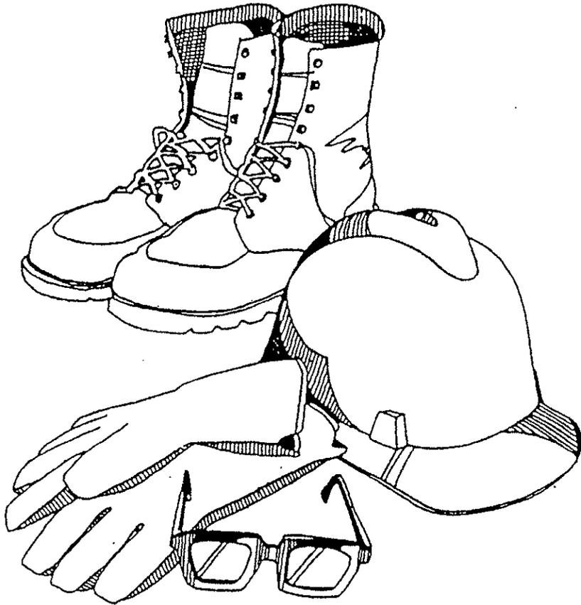
When drilling is performed in chemically or radiologically contaminated ground, special protective equipment and clothing may, and probably will, be required. The design and composition of the protective equipment and clothing must be determined jointly by the management and the client who requests the drilling services, and under some circumstances, with the concurrence of a health and safety professional.
