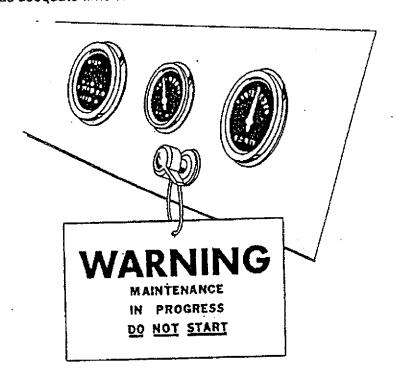
Never climb the mast (derrick) to do maintenance or make repairs. Lower mast, stop engine and deenergize rig before starting maintenance or repair on mast.
