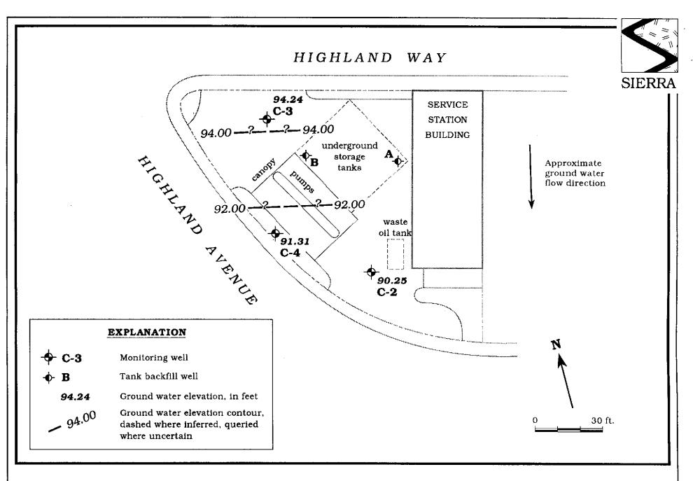
Figure 2. Monitoring Well Locations and Ground Water Elevation Contour Map - January 6, 1993 - Chevron Service Station #9-0329, 340 Highland Avenue, Piedmont, California
