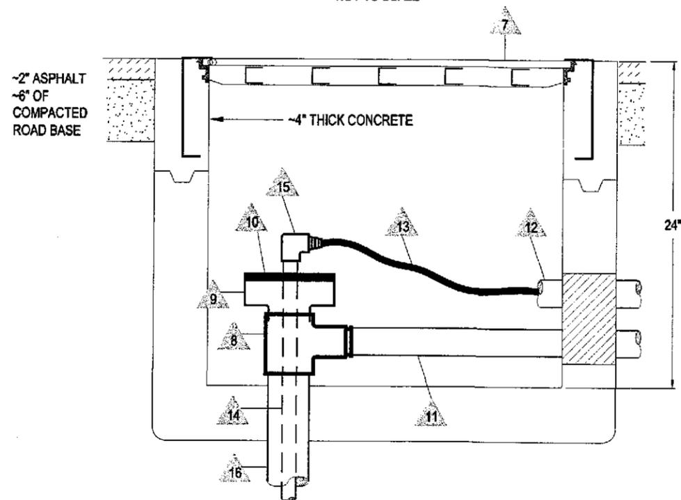
**Manifold System - Soil Vapor Extraction / Air Sparge Well Piping**
