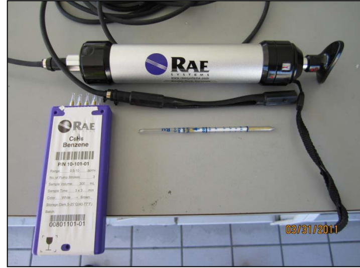
PHOTO 22: RAE System hand pump and benzene colorimetric tubes used for air monitoring during UST work.
