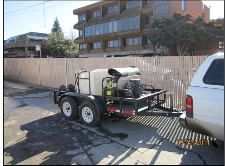
PHOTO 16: EnviroServ steam cleaning unit.
