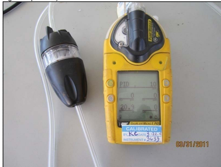
PHOTO 23: MicroGasAlert 5 meter used for monitoring air conditions and UST atmosphere during Site work. The 10 ppm PID reading is residual from having just been used inside the 15K UST.
