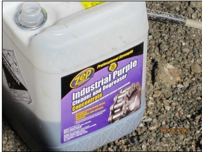
PHOTO 21: Detergent used during UST steam cleaning (5 gallons in total for both USTs). Four gallons of Simple Green was also used. (2-gallons per UST).
