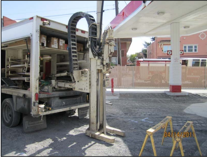
PHOTO 57: Collecting UST excavation confirmation soil samples, post backfill, using a GeoProbe 6600 direct push drill rig.
