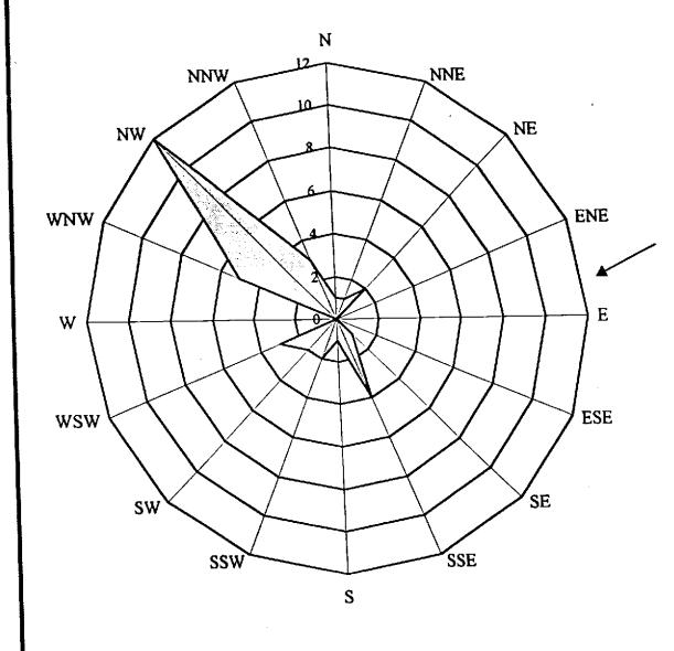
Number of monitoring events in which groundwater was reported to flow in a particular direction.
