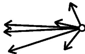
Rose diagram showing groundwater flow direction frequency, based on 12 episodes of monitoring from 12/93 to 1/00. Longer arrows represent more occurrences of that flow direction.
