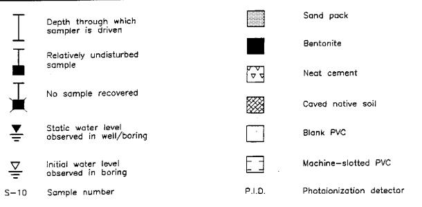
BLOWS REPRESENT THE NUMBER OF BLOWS OF A 140-POUND HAMMER FALLING 30 INCHES TO DRIVE THE SAMPLER THROUGH EACH 6 INCHES OF AN 18-INCH PENETRATION.
