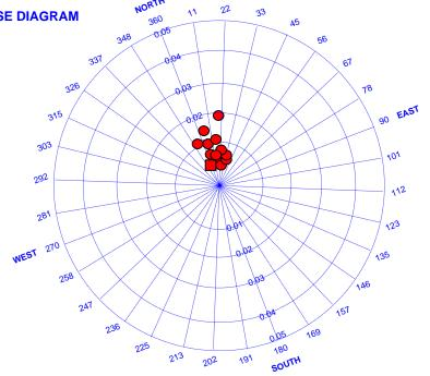
Rose diagram showing historic flow direction & gradient. Circles show historic data from six wells MW-1 to MW-6. Square shows most recent data from April 2009 using nine onsite monitor wells. Average of 14 flow direction measurements is approximately 16 degrees east of north.
