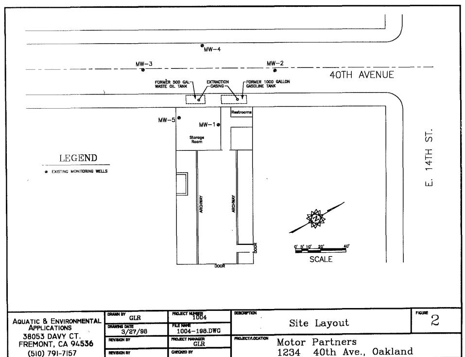
Sampling conducted on January 11, 1994 indicated levels of TPH-gasoline for the former waste oil tank area between 100 and 700 ppm. Levels of TPH-gasoline for the former gasoline tank area ranged from 150 to 1,200 ppm.
