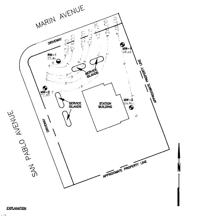
29.00 = Line of equal elevation of groundwater above mean sea level (MSL)
