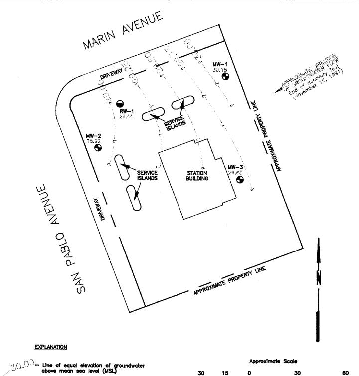
30.15 = Elevation of groundwater in feet MSL, end of recovery test, November 15, 1991
