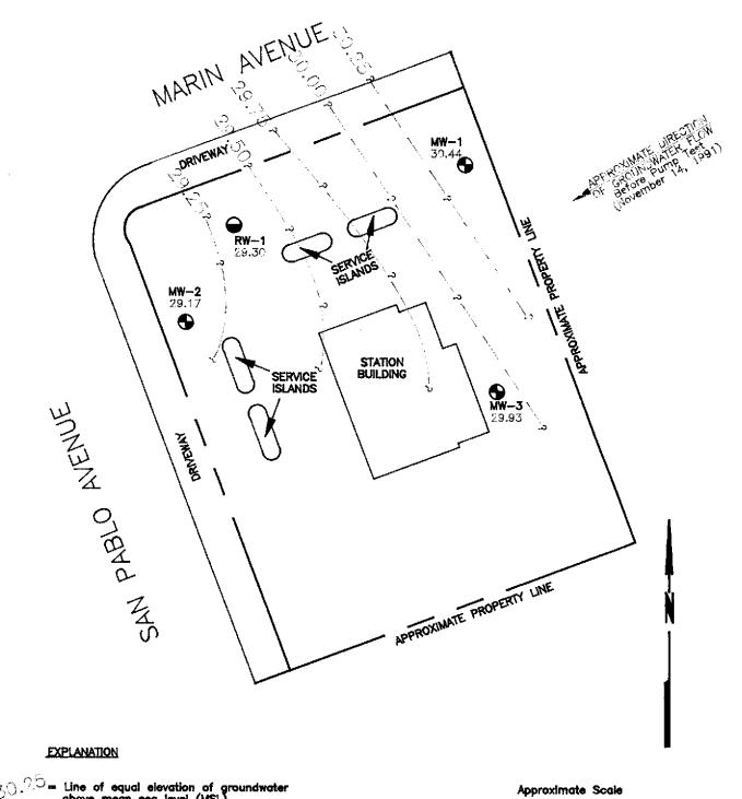
30.25 = Line of equal elevation of groundwater above mean sea level (MSL)
