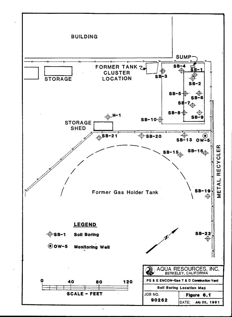
6.1.2 Welding Shop - In April and May 1991, ARI investigated soils beneath the welding shop. The goal of this effort was to determine the horizontal extent of elevated levels of petroleum hydrocarbons in soil. Previous investigations performed by PG&E found elevated levels of hydrocarbons in the vicinity of the building which were suspected of also being present under the building.
