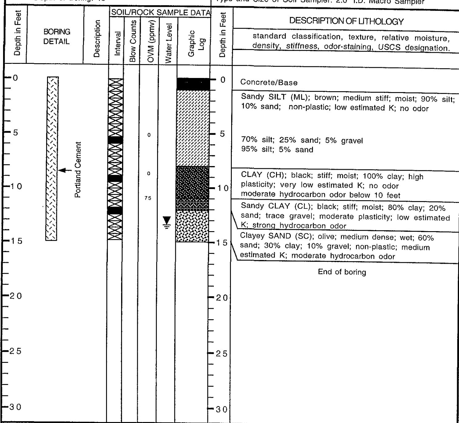
**SOIL BORING LOG AND MONITORING WELL COMPLETION DETAILS**
