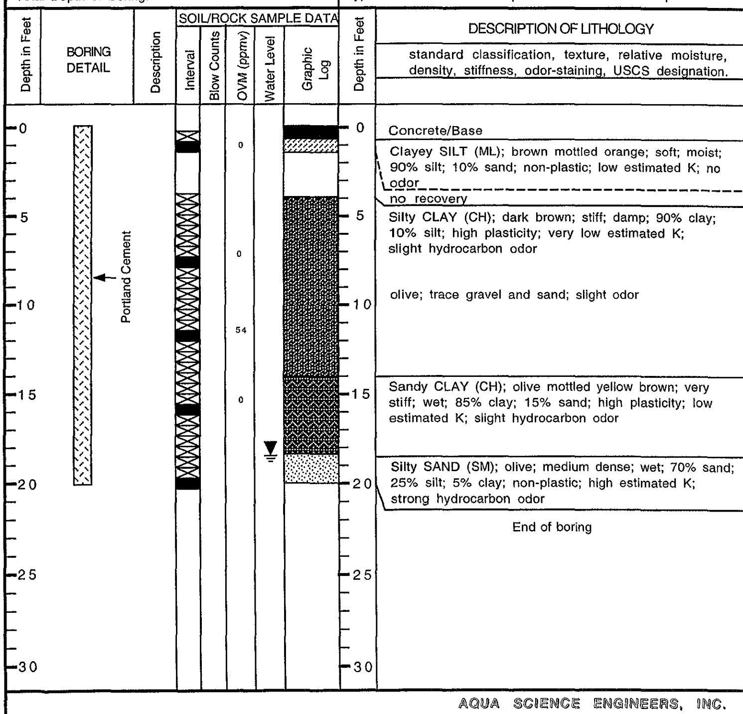
**SOIL BORING LOG AND MONITORING WELL COMPLETION DETAILS**
