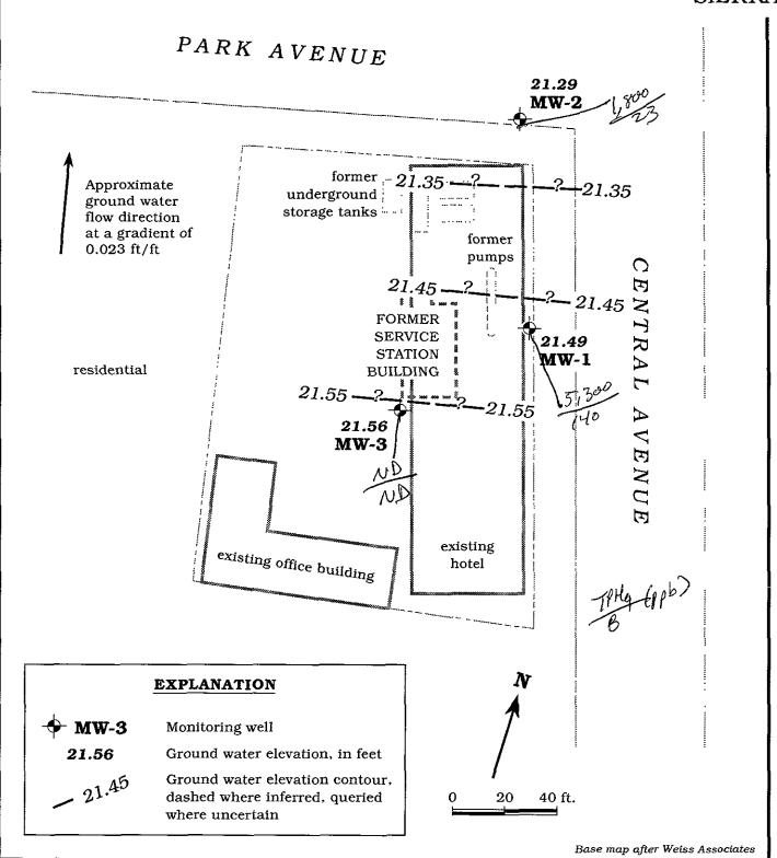
Figure 1. Monitoring Well Locations and Ground Water Elevation Contour Map - June 21, 1994 - Former Chevron Service Station #9-0100, 2428 Central Avenue, Alameda, California
