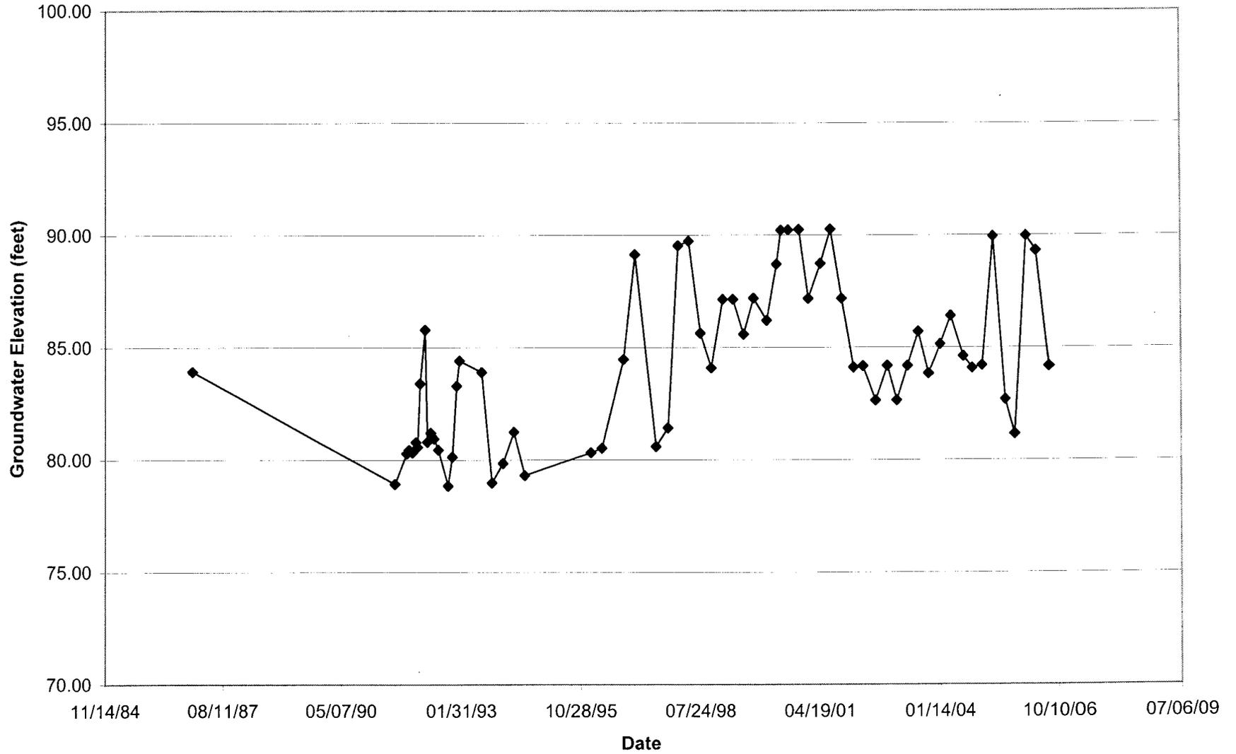
MW-3 Groundwater Elevation vs. Time
