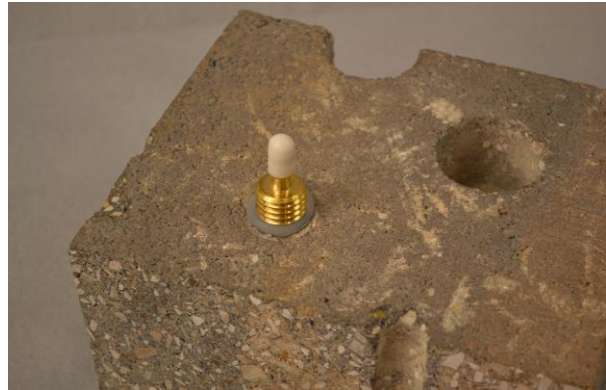
Figure 3. Installed VAPOR PIN®
