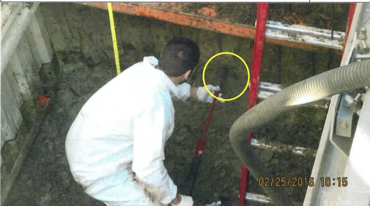
DESCRIPTION: COLLECTING NORTH WALL SOIL SAMPLE 8 FT FROM SURFACE
