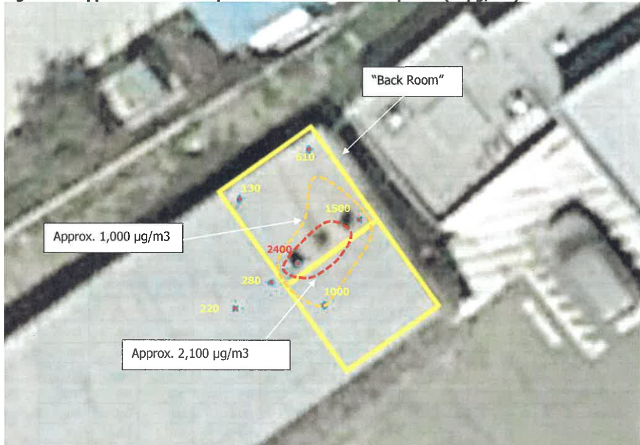
Figure 3 – Approximate Soil Vapor PCE Concentration Isoleths (in \mu\text{g}/\text{m}^3 )
