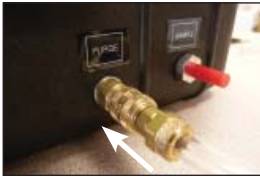
On the Large Vac-U-Chamber, grip the release ring and push toward the chamber.
