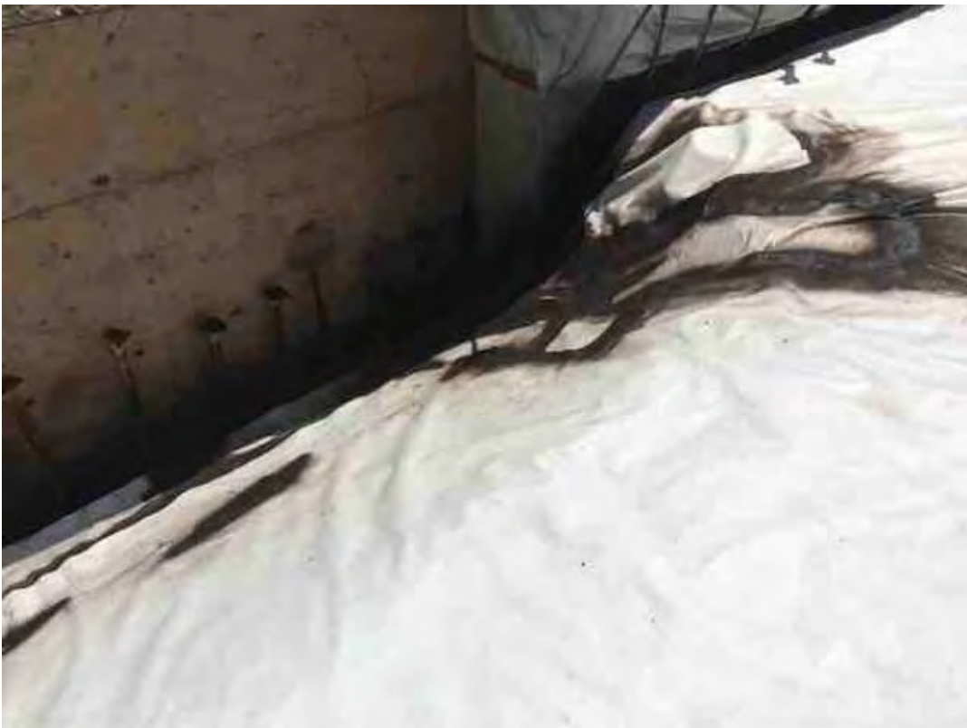
Smoke test. Lifted pad
