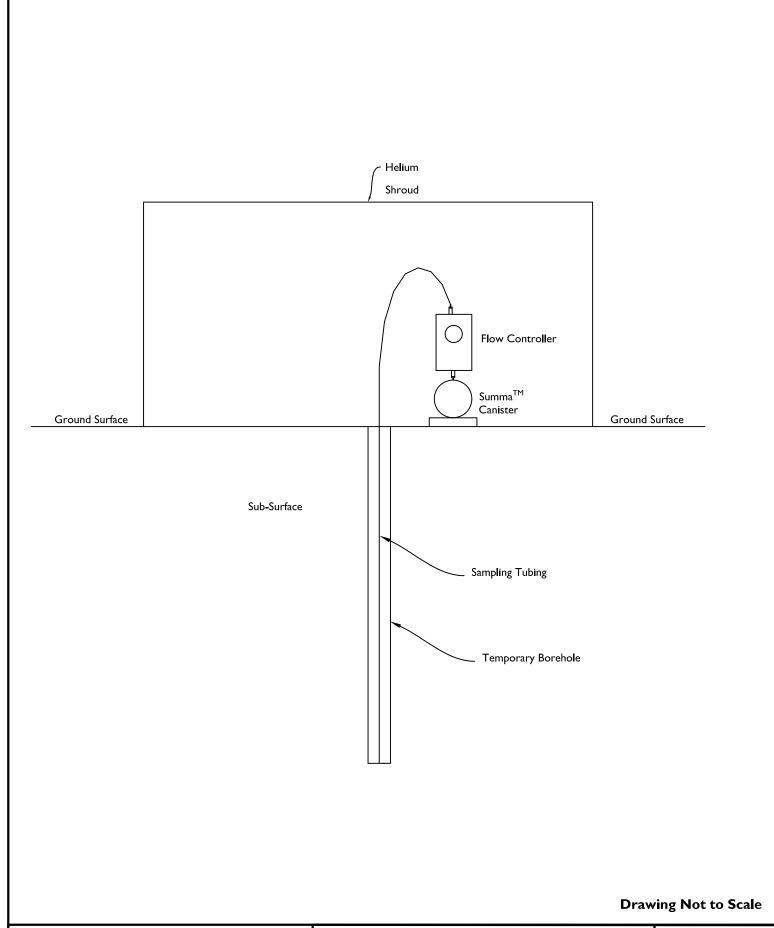
Soil Vapor Probe Sampling Train Diagram
