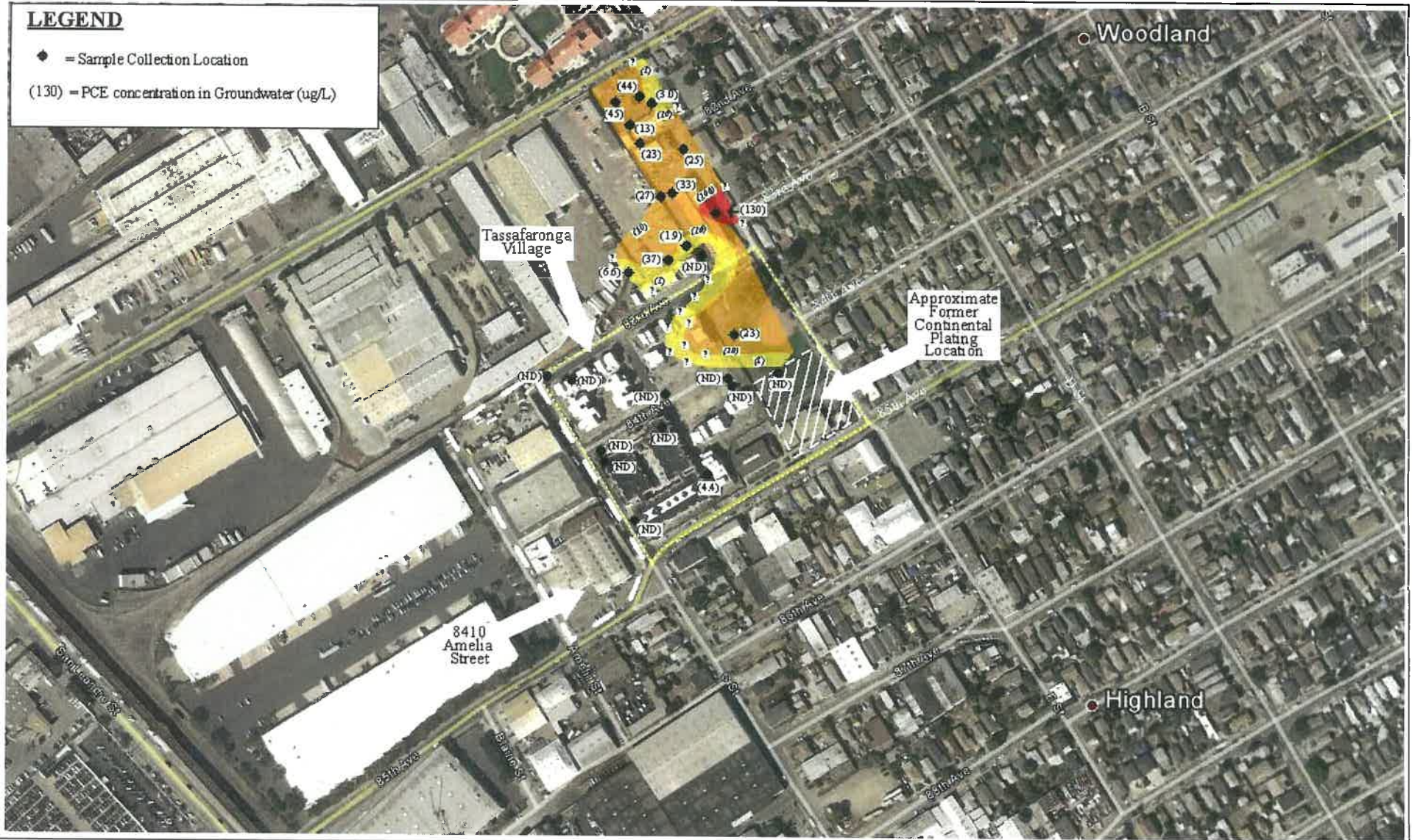
Figure Site Vicinity Map Showing PCE in Groundwater 8410 Amelia Street Oakland, California
