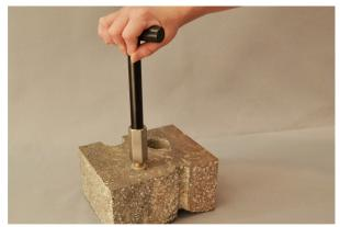
Figure 7. Removing the Vapor Pin<sup>TM</sup>.
