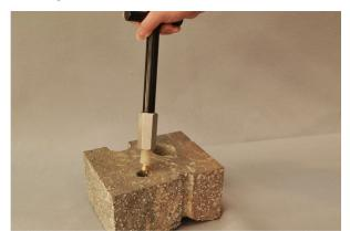
Figure 8. Extracted Vapor Pin<sup>TM</sup>.
