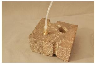
Figure 5. Vapor Pin<sup>™</sup> sample connection.
