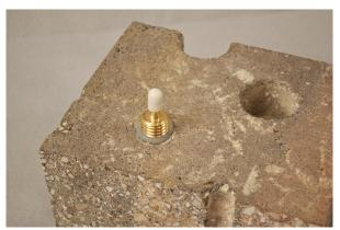
Figure 4. Installed Vapor Pin<sup>TM</sup>.
