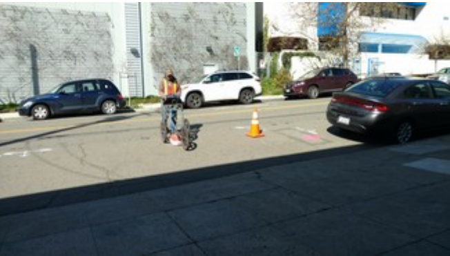
Photograph No. 11 – Northwest view from Webster Street sidewalk at Roll-Up door entrance to former service department showing Subtronic Corporation using Ground Penetrating Radar equipment to assess presence of subsurface utilities beneath parking lane (WGE, 3/1/17).
