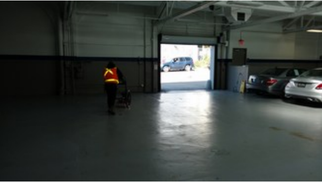
Photograph No. 10 – Northwest view from interior of former Mercedes-Benz Service Department showing Subtronic Corporation using Ground Penetrating Radar equipment to assess presence of subsurface utilities beneath concrete slab floor (WGE, 3/1/17).
