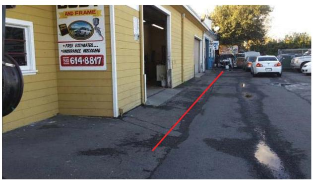
The red line above represents the path of one of the many scans; the GPR data for this particular scan is shown below.
