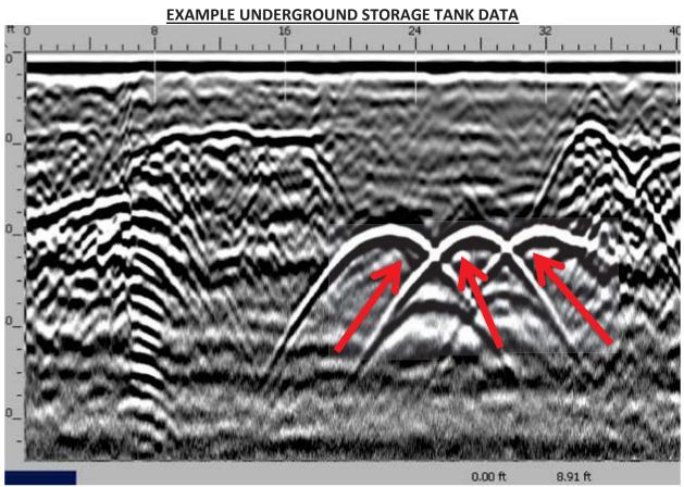
The above GPR data screen shot shows a scan across 3 tanks. The red arrows are pointing out these reactions. This scan was taken from a <u>different site</u> and is shown here as an example of how UST's might appear had they been found.
