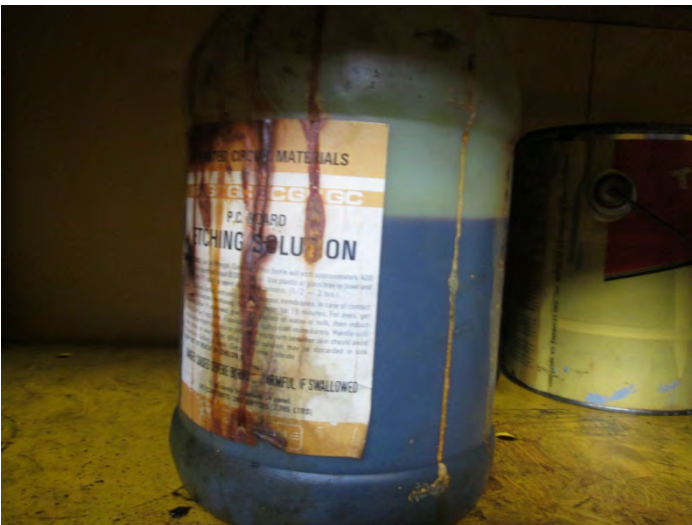
23. Container labelled "P.C. Board Etching Solution" found in hazardous substances closet #2, with staining around outside of container
