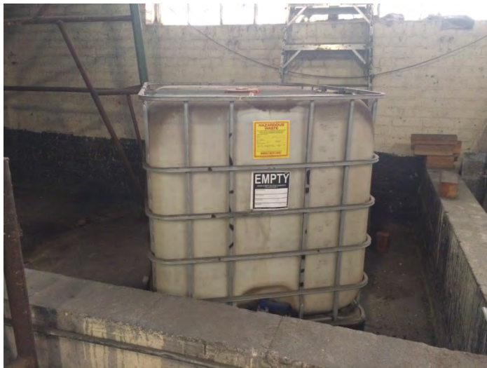
11. Empty hazardous waste tote with secondary containment, located in east side of warehouse
