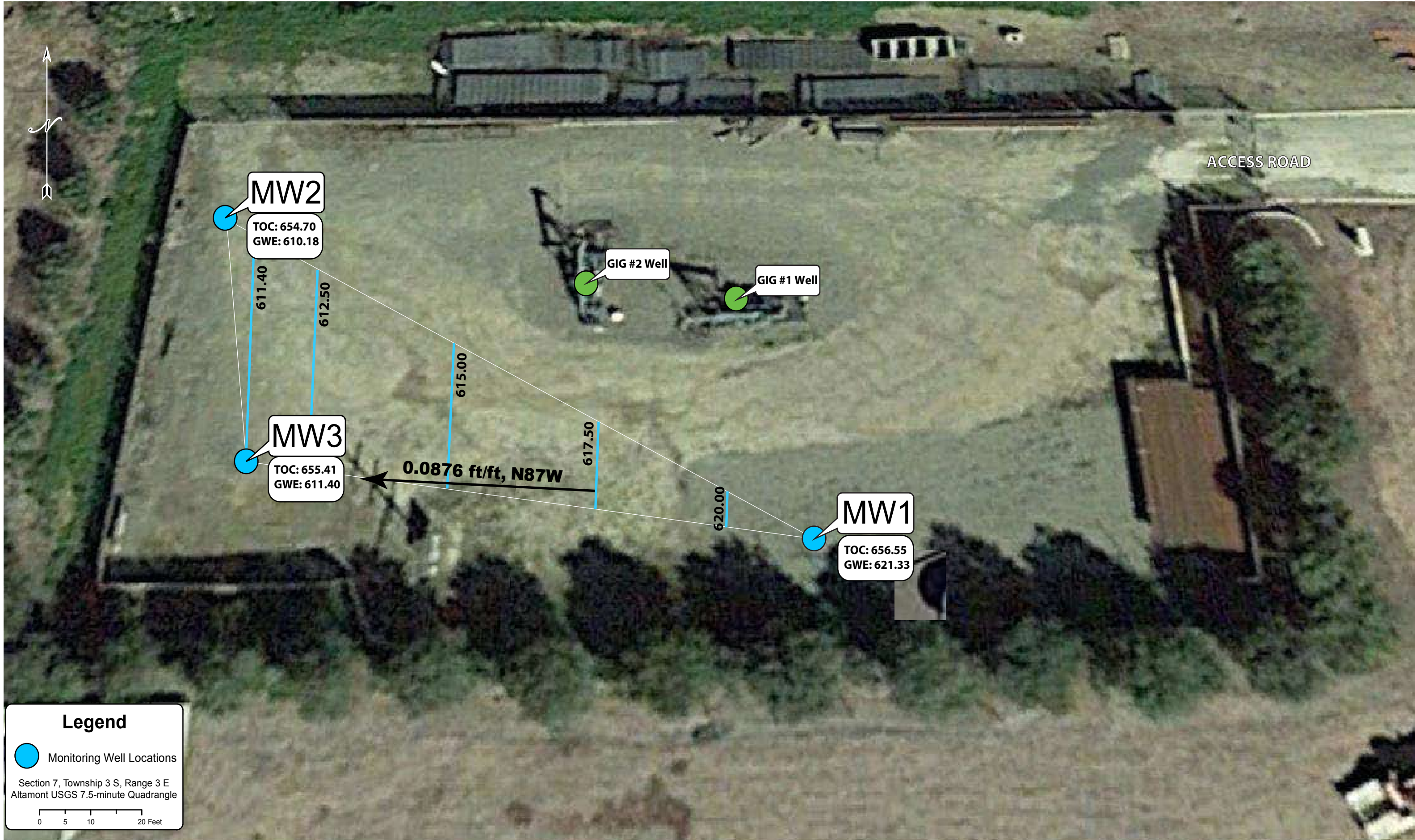
FIGURE 5 Monitoring Well Location and Groundwater Gradient Map
