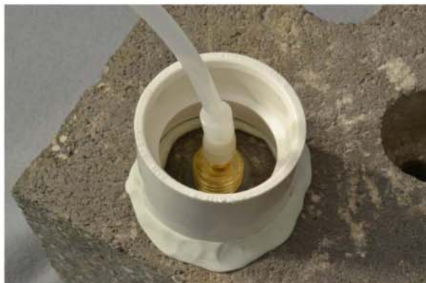
Figure 6. Water dam used for leak detection.
