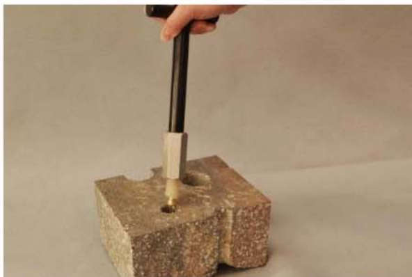
Figure 8. Extracted Vapor Pin™.
