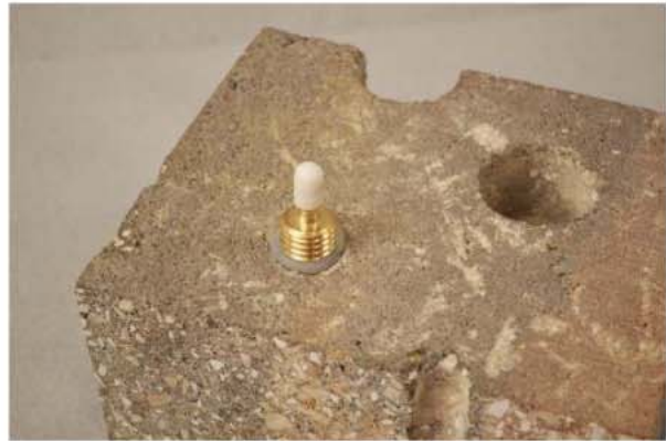
Figure 4. Installed Vapor Pin™.
