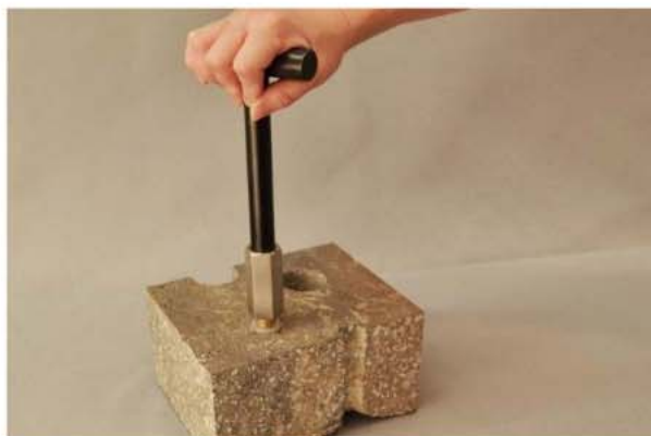
Figure 7. Removing the Vapor Pin™.
