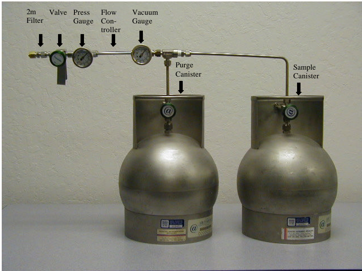
Figure 4, Sampling Manifold Set-up.
