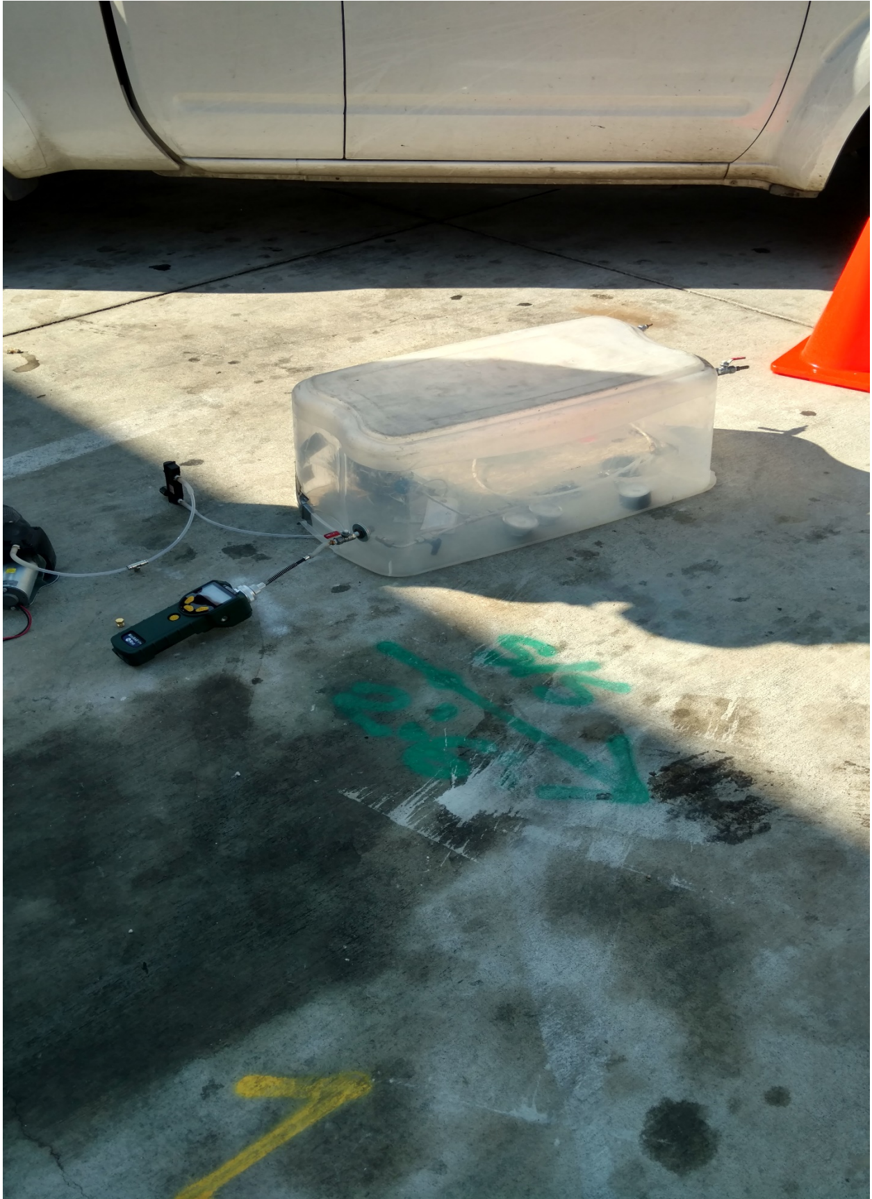
Figure 5 - Sampling Shroud with 1-Liter SUMMA® Canister/Manifold and PID Meter to Monitor Tracer Gas Concentration
