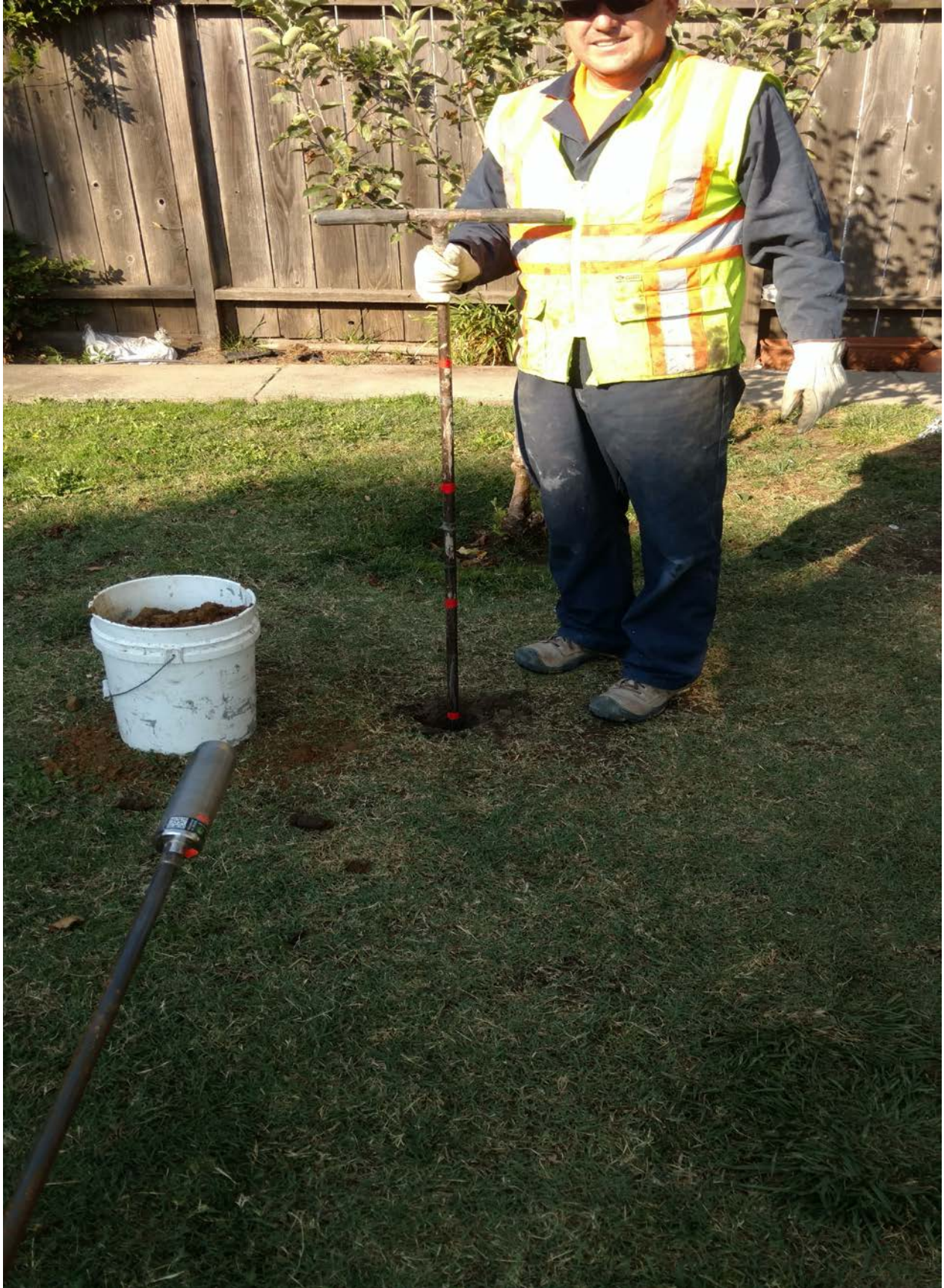
Drilling SB-7 with Hand Auger Figure 6
