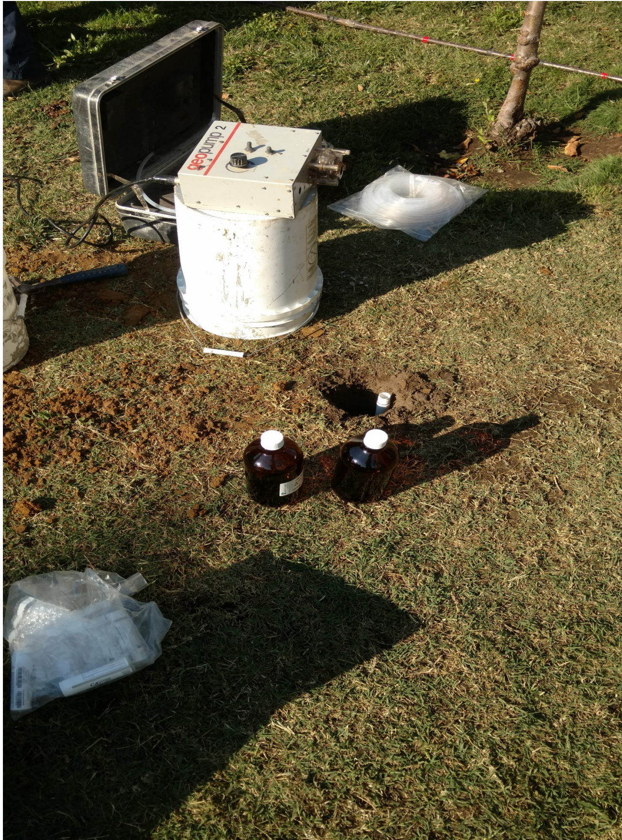
Collecting Water Samples from Boring SB-7 Figure 6A
