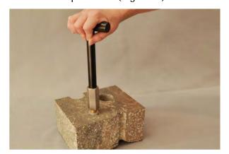
**Figure 7**. Removing the Vapor Pin<sup>TM</sup>.
