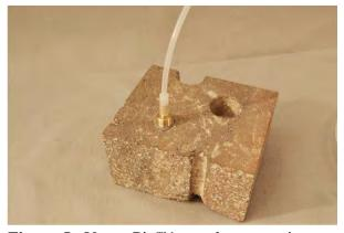
**Figure 5**. Vapor Pin<sup>TM</sup> sample connection.
