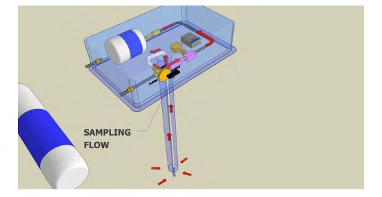
**Figure 4: Sampling Flow Diagram**
