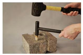
**Figure 2**. Installing the Vapor Pin<sup>TM</sup>.
