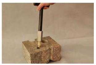
Figure 8. Extracted Vapor Pin<sup>TM</sup>.
