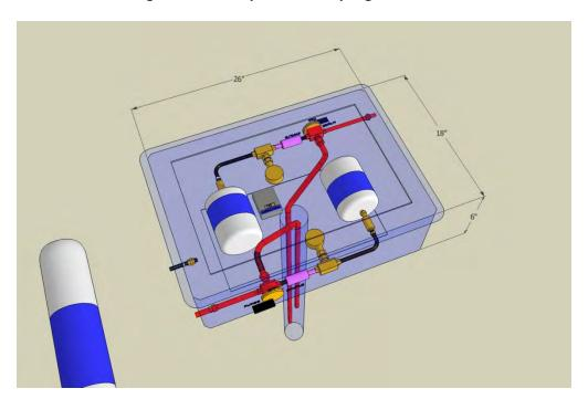
Figure 5: Dual Depth Well Sampling Shroud
