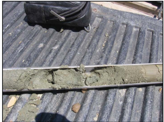
Photograph 4: A green-stained, moist, silty-sand layer was encountered in soil boring B1 at approximately 13.5 ft bgs.
