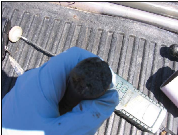
Photograph 3: As seen in the background, a photo-ionization detector was used to screen soil, groundwater and ambient air for VOCs.
