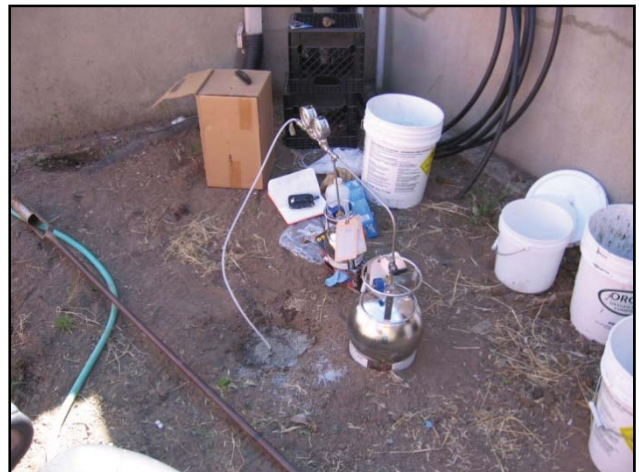
Photograph 6: The soil vapor sampling set-up for soil vapor sample SV-4. Isopropyl was used as a tracer.
