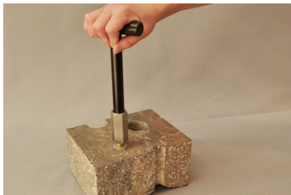
Figure 7. Removing the Vapor Pin™.
