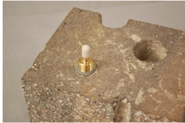
Figure 4. Installed Vapor Pin™.
