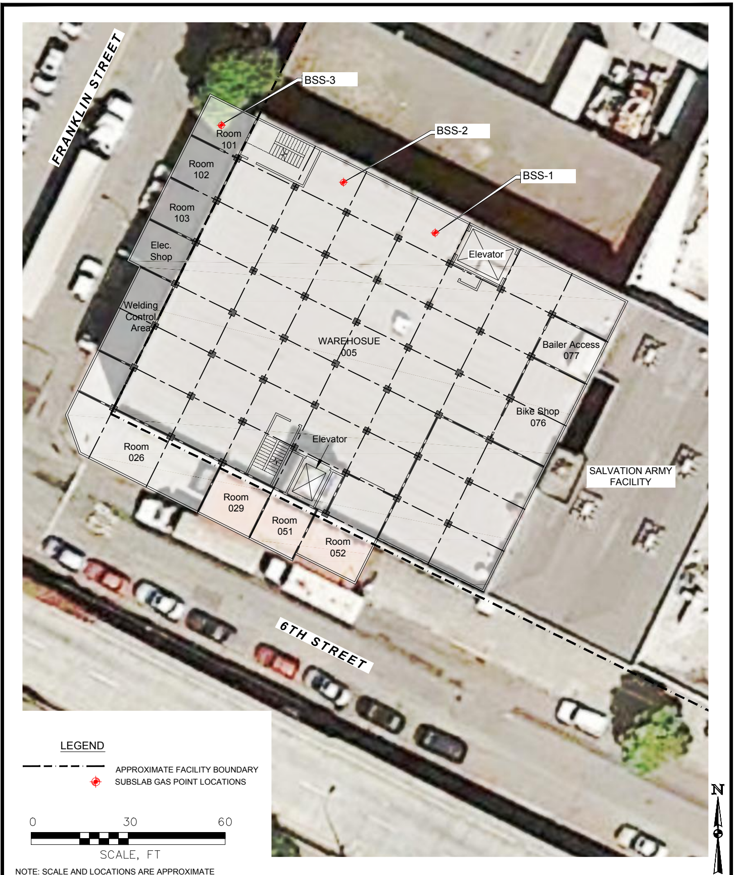
FIGURE 8 Subslab Soil Gas Sampling Point Locations THE SALVATION ARMY 601 WEBSTER STREET OAKLAND, CALIFORNIA
