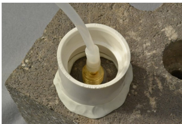
Figure 6. Water dam used for leak detection.
