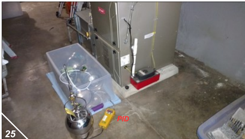
Photograph Nos. 22-27 - Views of sub-slab vapor sampling activities at Field Sampling Point SS1 located within existing furnace room in basement; Field Point SS1 installed next to former oil burner and product lines associated with UST; Photograph Nos. 22 & 24 shows initial sub-slab vacuum (0.000"Hg) and interior shroud VOC measurement (376 ppm) during sampling with Summa canisters; Photograph Nos. 23 & 25 show sub-slab vapor sampling in progress, with typical manifold assembly, shroud enclosure, and measurement of shroud tracer gas (2-Propanol) using calibrated PID; Photograph Nos. 26 & 27 show subsequent sub-slab sampling for TPH-Diesel & Naphthalene (TO-17) using Thermal Desorption Tubes (In series) and sampling pump (WGE, 2/1/18).
