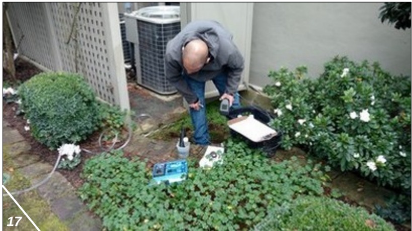
Photograph Nos. 17 & 18 – Respective southeast and west views of residence at 125 Guilford Road showing Dysert Environmental field technician during purging/monitoring/sampling of private water supply well; sample collected directly from effluent spigot located approximately 13 feet west of wellhead shown in Photograph No. 18; private water supply well installed in February 2016 by Martell Water Systems, Inc. to depth of 200 feet (WGE, 1/18/18).
