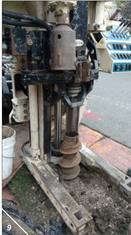
Photograph Nos. 8 & 9 – Respective northeast and southeast views of front yard and sidewalk of subject residence, showing EnProbe Drilling personnel during rotary hollow stem auger drilling at Field Point B3, located approximately 7 feet south of former UST excavation, and in direct vicinity of former UST remote fill pipe; Photograph No. 9 shows GeoProbe sampler advanced through center of hollow stem augers during collection of discrete soil samples in bedrock zone at 10 and 14 fbg; borehole drilled to total depth of 14 fbg (WGE, 1/18/18).
