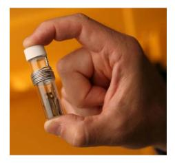
Figure 2 - PSG Sampler
