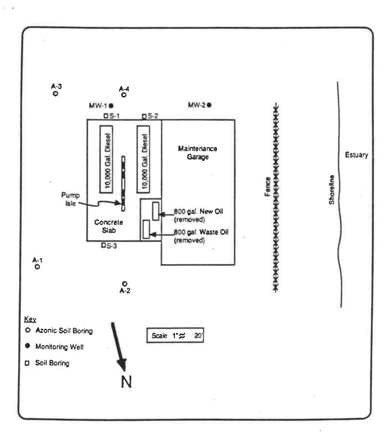
Figure 2. Location of Monitoring Wells and Soil Borings
