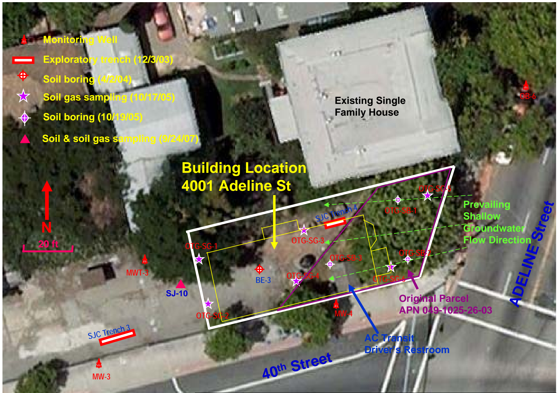
09EMV03.1000 May 21, 2009 Figure 3. Site Plan with Identification of Sampling Locations 4001 Adeline Street, Emeryville, California (Parcel APN 049-1025-26-03)
